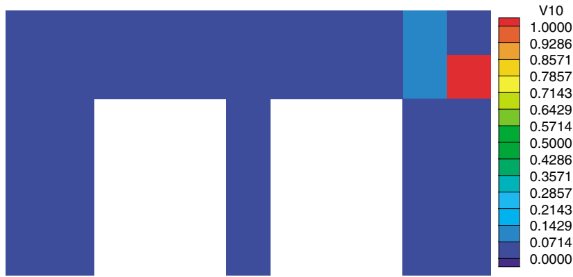
Fig. 20. Example 4: normalized distribution of local error indicator \beta_k .
