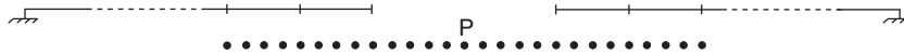
Figure 32. Coupling between the particle and the continuum model in the Arlequin framework.
